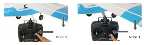
23. Open the throttle slowly and check that the motor shaft turns in an anticlockwise direction (when viewed from the front).
