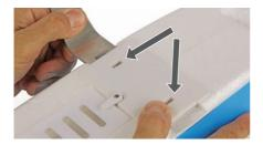
Insert the undercarriage nose leg into the joiner tube, position the flat section of the leg directly behind the Allen screw, then securely tighten the screw to clamp the leg in place.
