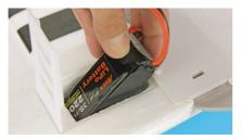
12. Remove the KA-6 transmitter battery cover and insert four AA alkaline cells (not included) taking care to observe the correct polarity.
